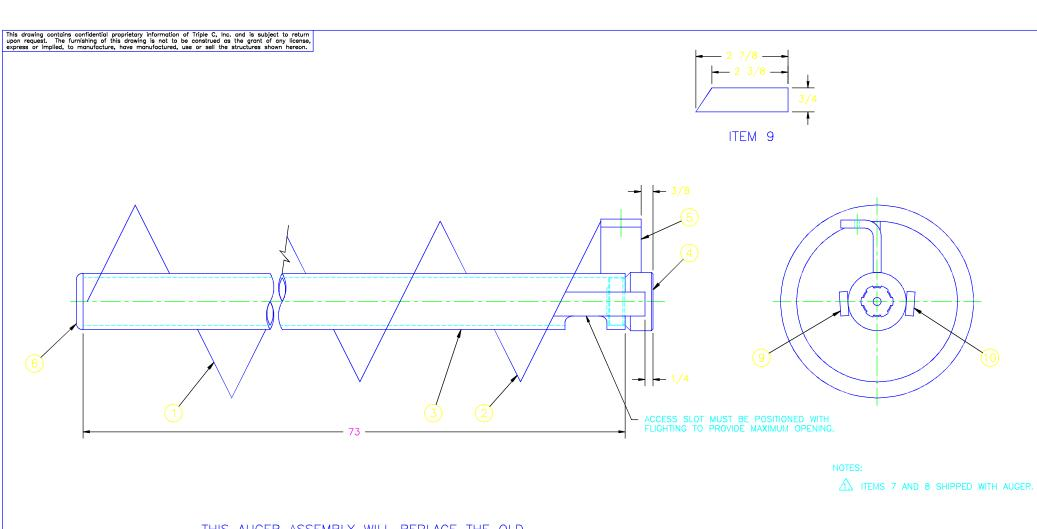
THIS AUGER ASSEMBLY WILL REPLACE THE OLD STYLE AUGER PREVIOUSLY HELD IN BY 1/4" ROD.
